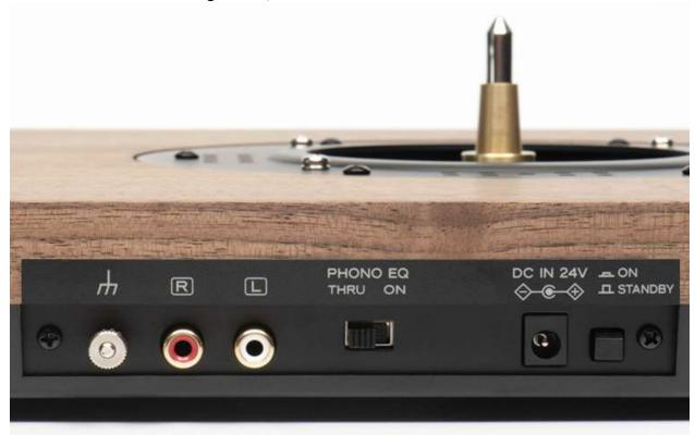
The back panel is fairly well populated. First comes the ground/earth connection, followed by a pair of RCA output jacks and a switch for activating or defeating the onboard phono stage. That switch has two positions: On, which means the phono stage is active, and Thru, which means it's out of the circuit and the turntable should be connected to the phono input of an amplifier. Finally, there's the input for the 24V DC power supply and, next to it, the power standby/on switch.
