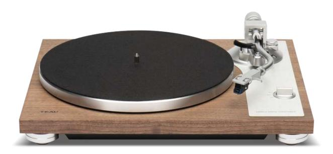
Significantly, it's a direct-drive design. Direct-drive 'tables have regained much of the popularity they enjoyed in the 1970s and '80s. TEAC claims the TN-4D-SE's brushless, quartz-controlled DC servo motor banishes cogging—the rapid, jerky rotation of the direct-drive motor—which was
